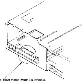
Former type: Eject motor (M601) is invisible. New type : Eject motor (M601) is visible.
